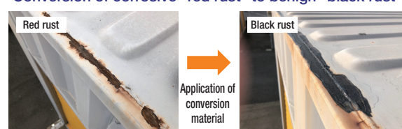
Conversion of corrosive “red rust” to benign “black rust”
